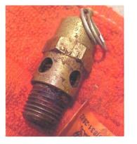
B. On receipt inlet of 125 psig valve is clogged with debris
