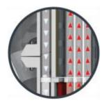
*Gravity* – colder (denser) primary coolant "falls" to bottom of reactor pressure vessel, cycle continues
