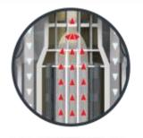
**Convection** – energy from the nuclear reaction heats the primary reactor coolant causing it to rise by convection and natural buoyancy through the riser, much like a chimney effect
