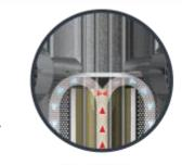
**Conduction** – heat is transferred through the walls of the tubes in the steam generator, heating the water (secondary coolant) inside them to turn it to steam. Primary water cools.
